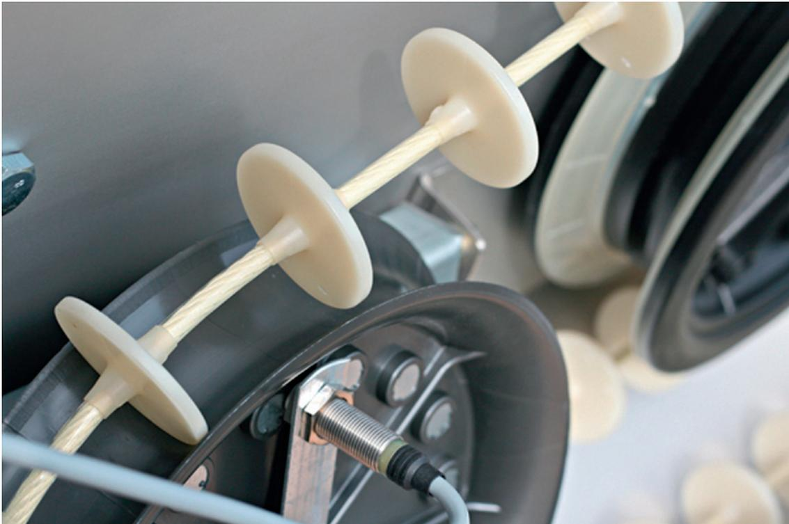
◀ Friction wheel transfers the drive of the motor of 0.75 kW
